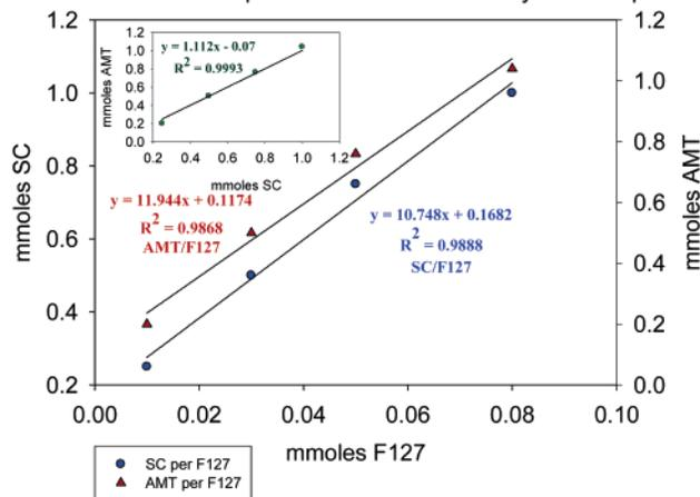
**Figure 7.** Optimal binding ratio of SC to F127 in microemulsions (shown by blue points) and optimal binding ratio of AMT to F127 (shown by red points). The inset shows the binding ratio of SC to AMT.
