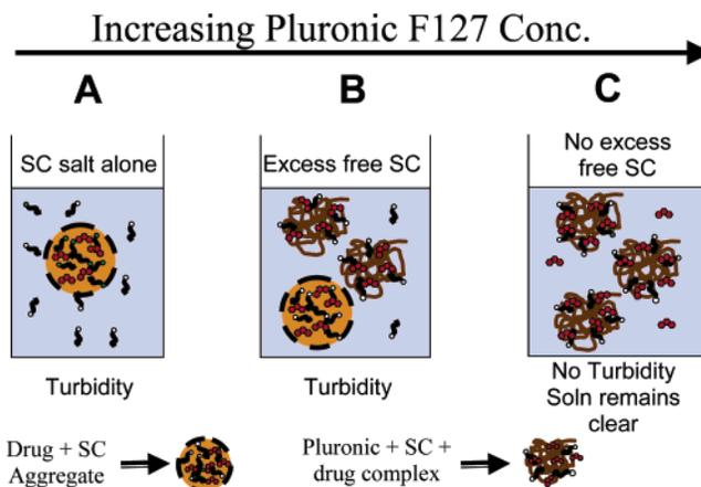
**Figure 4.** Schematic diagram of turbidity in various solutions. Surfactants with green heads represent the sodium caprylate. The red three-ring structure represents the amitriptyline drug. Black coils represent Pluronic F127. The light blue agglomerate system represents the complex that is formed between the free (monomeric) sodium caprylate in the bulk and the amitriptyline. This complex formation causes turbidity to appear in the system.
