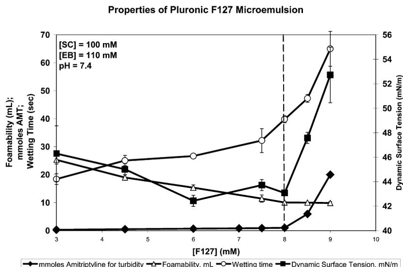
**Figure 6.** Graph of the turbidity, foamability, fabric wetting time, and dynamic surface tension of microemulsion systems with the SC concentration fixed at 100 mM, the EB concentration fixed at 110 mM, and varied F127 concentrations.
