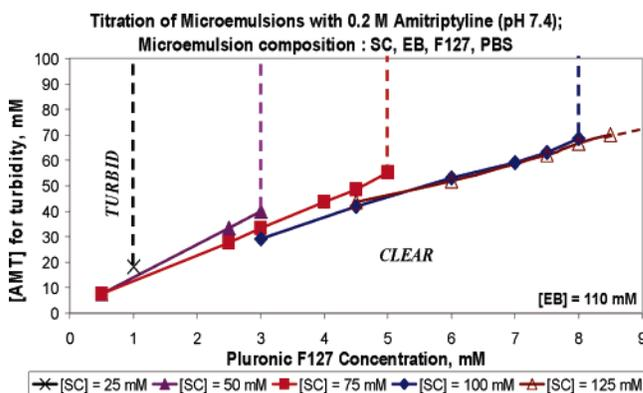
**Figure 5.** Titration of microemulsion systems with AMT. The sodium caprylate concentration is varied from 25 to 125 mM, and the F127 concentration is varied from 1 to 9 mM. The solution is clear in the area below the curve and turbid in the area above the curve.
