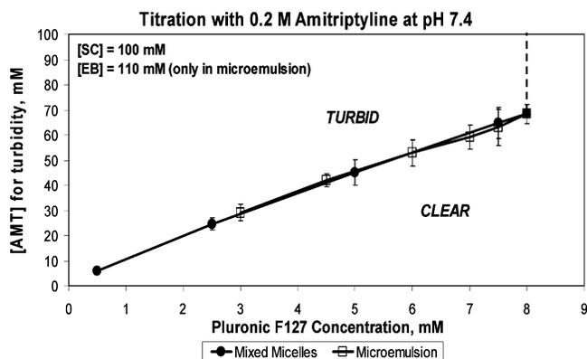
**Figure 3.** Titration of mixed micelles and microemulsion systems. The solution is clear in the area below the curve and turbid in the area above the curve.
