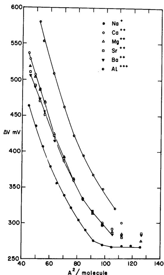
FIG. 4. Surface potential-area curves of synthetic (dipalmitoyl) lecithin on subsolutions of 0.02 M NaCl + 0.01 M metal salt ( $\text{CaCl}_2$ ,  $\text{MgCl}_2$ ,  $\text{SrCl}_2$  or  $\text{BaCl}_2$ ) at pH 5.6 and  $\text{Al}(\text{NO}_3)_3$  at pH 3.8 and 25°.
