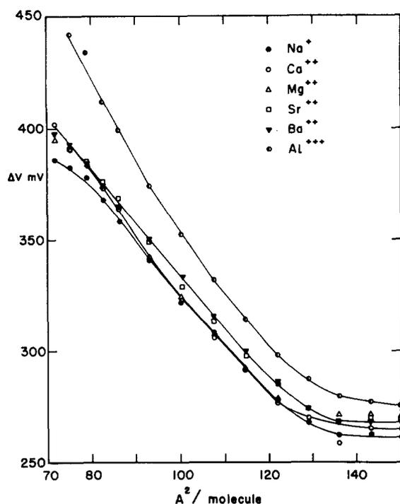
FIG. 6. Surface potential-area curves of yeast lecithin on subsolutions of 0.02 M NaCl + 0.01 M metal salt ( $\text{CaCl}_2$ ,  $\text{MgCl}_2$ ,  $\text{SrCl}_2$  or  $\text{BaCl}_2$ ) at pH 5.6 and  $\text{Al}(\text{NO}_3)_3$  at pH 3.8 and  $25^\circ$ .
