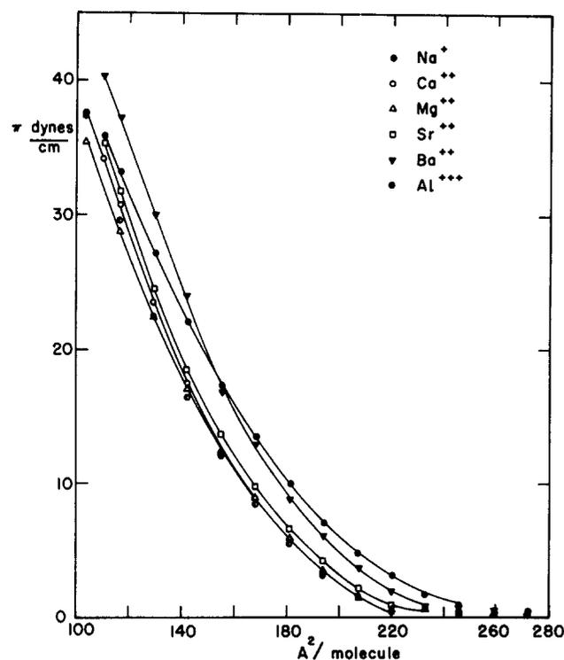
FIG. 13. Surface pressure–area curves of cardiolipin on subsolutions of 0.02 M NaCl + 0.01 M metal salt ( $\text{CaCl}_2$ ,  $\text{MgCl}_2$ ,  $\text{SrCl}_2$  or  $\text{BaCl}_2$ ) at pH 5.6 and  $\text{Al}(\text{NO}_3)_3$  at pH 3.8 and  $25^\circ$ .
