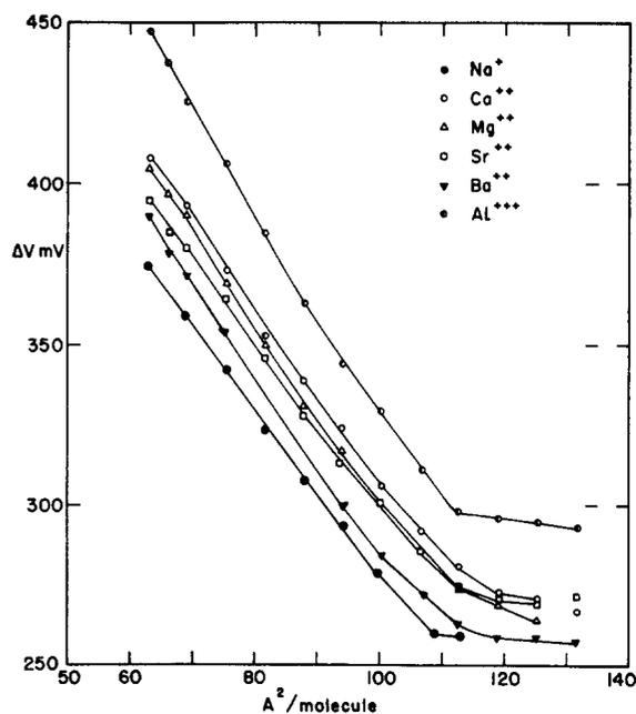
FIG. 5. Surface potential-area curves of egg lecithin on subsolutions of 0.02 M NaCl + 0.01 M metal salt ( $\text{CaCl}_2$ ,  $\text{MgCl}_2$ ,  $\text{SrCl}_2$  or  $\text{BaCl}_2$ ) at pH 5.6 and  $\text{Al}(\text{NO}_3)_3$  at pH 3.8 and 25°.
