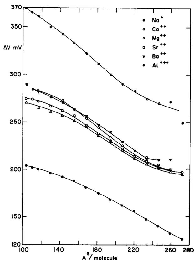
FIG. 14. Surface potential–area curves of cardiolipin on subsolutions of 0.02 M NaCl + 0.01 M metal salt ( $\text{CaCl}_2$ ,  $\text{MgCl}_2$ ,  $\text{SrCl}_2$  or  $\text{BaCl}_2$ ) at pH 5.6 and  $\text{Al}(\text{NO}_3)_3$  at pH 3.8 and  $25^\circ$ .
