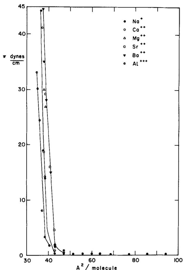
FIG. 9. Surface pressure-area curves of dicetyl phosphate on subsolutions of 0.02 M NaCl + 0.01 M metal salt ( $\text{CaCl}_2$ ,  $\text{MgCl}_2$ ,  $\text{SrCl}_2$ , or  $\text{BaCl}_2$ ) at pH 5.6 and  $\text{Al}(\text{NO}_3)_3$  at pH 3.8 and  $25^\circ$ .
