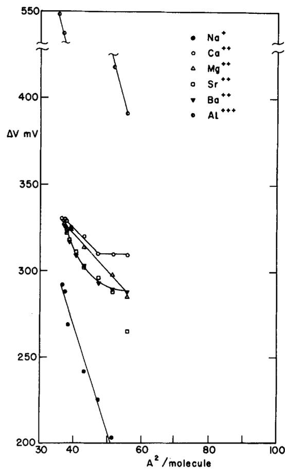
FIG. 10. Surface potential-area curves of dicetyl phosphate on subsolutions of 0.02 M NaCl + 0.01 M metal salt ( $\text{CaCl}_2$ ,  $\text{MgCl}_2$ ,  $\text{SrCl}_2$ , or  $\text{BaCl}_2$ ) at pH 5.6 and  $\text{Al}(\text{NO}_3)_3$  at pH 3.8 and  $25^\circ$ .
